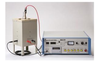
Figure 7. Stand-mounted coil for application of uniform magnetic field
