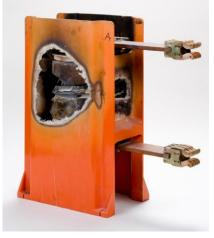
Figure 5. Failed vacuum interrupter
