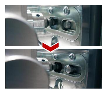
6. Rotate the latch handle on the back of the Remote Operator to the locked position to latch it in place.
