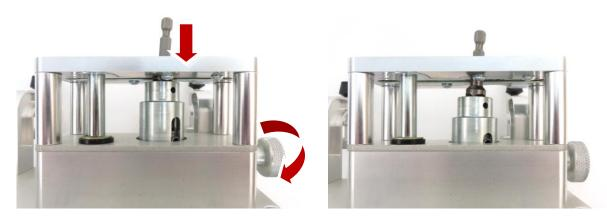
5. With the latch handle on the Remote Operator in the unlocked position, align the pins on the SecureConnect plug-in unit to the holes on the SecureConnect Remote Operator, and slide the Remote Operator onto the plug-in unit, over the pins.
