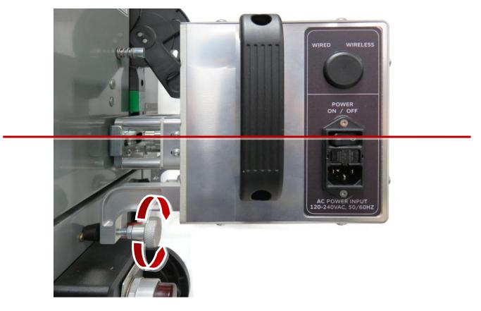
9. Pull out and turn the knurled locking knob on the right-hand side of the Remote Operator and rotate it 90° to release the ¼" tool head. Release the handle for the CENTERLINE 2100 unit.
